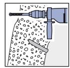
Bohren in Beton
